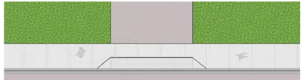
Driveway Crossing of Non-Separated Sidewalk (Wrapped Around Driveway)
