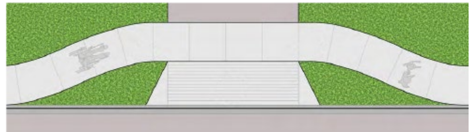
Driveway Crossing of Non-Separated Sidewalk (Wrapped Around Driveway)
