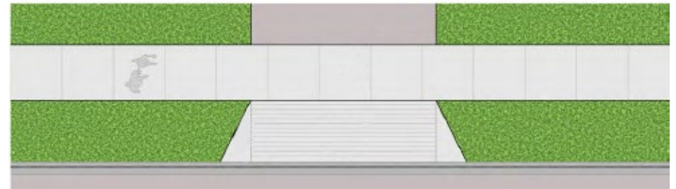
Driveway Crossing of Non-Separated Sidewalk
